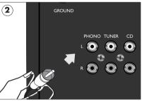
Connect the **LEFT** lead from your record turntable to the socket marked **PHONO** and **L**.
