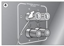
To connect each speaker wire, loosen the terminal by turning anticlockwise. Wrap the bare wire around the metal terminal. Tighten in a clockwise direction.
