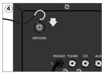
If your turntable is the type which has a separate earth or ground lead, connect this lead to the fitting marked **GROUND**.
