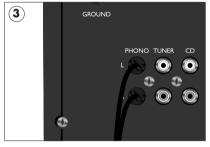
Connect the **RIGHT** lead from your record turntable to the socket marked **PHONO** and **R**.
