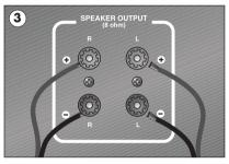
Connect the speaker cable from your left-hand speaker to the terminals marked **L**. The red wire goes to the red (+) terminal and the black wire goes to the black (-) terminal.
