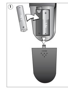
Slide open the battery compartment door by gently pressing in the direction of the arrow. Insert 2 AAA (LR03/MN2400) size batteries. Make sure you insert the batteries correctly. (as illustrated). Replace the compartment door.
