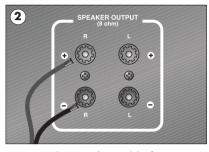
Connect the speaker cable from your right-hand speaker to the terminals marked  $\mathbf{R}$ . The red wire goes to the red (+) terminal and the black wire goes to the black (-) terminal.
