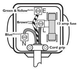
The wire which is coloured **Blue** must be connected to the terminal in the plug which is marked with the letter **N** or coloured **Black**.
