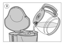
Fill the water reservoir to the maximum level (12) with cold water. Do not overfill.
