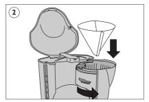
Swing out the filter holder and insert a suitable filter paper into the filter cone.
