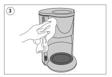
The body of the unit should be cleaned using a cloth dampened with warm water.
