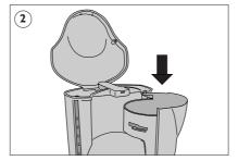
Replace the holder by inserting the pivot and lowering into position.
