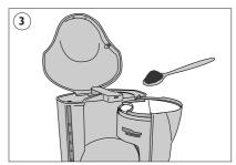
Put the measured quantity of coffee into the filter paper and close the holder.
